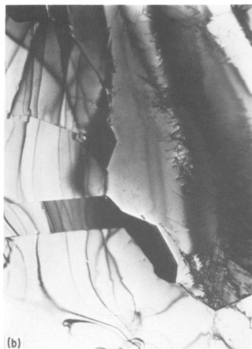
Figure 8 Transmission electron micrographs of duplex alloy aged for 5 min after deformation to a strain of 0.8 at 900°C at strain rates of (a) 1 and (b) 0.01 sec -1 . Recrystallized twinned austenite grains and dark sigma lie at the phase boundaries. × 82 000.
