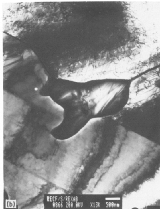
Figure 7 Transmission electron micrographs of samples aged for 5 min at 900°C after deformation to a strain of 0.8 at strain rates of (a) 1 and (b) 0.01 sec -1 . Ferrite is well recovered and austenite appears twinned within its grains. Dark particles of sigma can be seen at ferrite-austenite boundaries. × 56 000.
