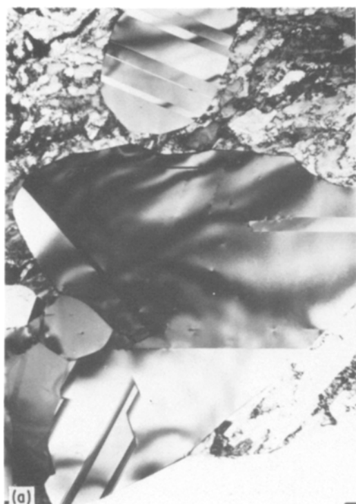
Figure 8 Transmission electron micrographs of duplex alloy aged for 5 min after deformation to a strain of 0.8 at 900°C at strain rates of (a) 1 and (b) 0.01 sec -1 . Recrystallized twinned austenite grains and dark sigma lie at the phase boundaries. × 82 000.
