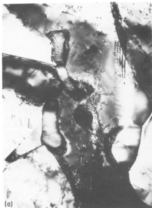
Figure 7 Transmission electron micrographs of samples aged for 5 min at 900°C after deformation to a strain of 0.8 at strain rates of (a) 1 and (b) 0.01 sec -1 . Ferrite is well recovered and austenite appears twinned within its grains. Dark particles of sigma can be seen at ferrite-austenite boundaries. × 56 000.
